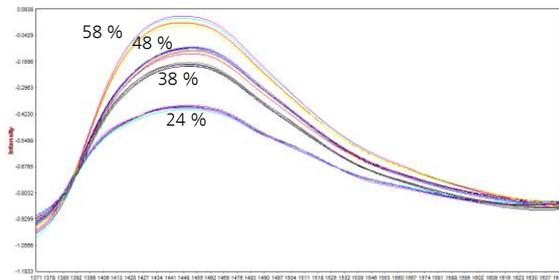
Figure 2: NIR spectra (with SNV) of the water absorption in soft contact lenses with 24%, 38%, 48%, and 58% embedded water.
