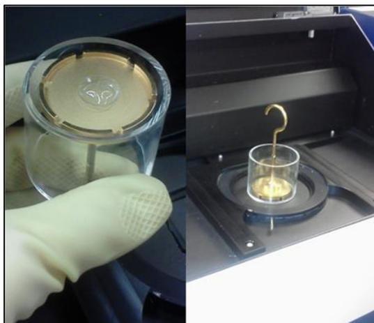
**Figure 1: The lens is centered on a diffuse gold reflector in a transflection vessel**
