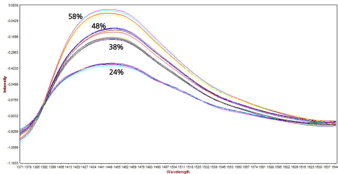
This application note describes the determination of water content in soft contact lenses by NIRS. Using a liquid sample kit with a gold diffuse reflector, the soft contact lenses were analyzed in transflection mode. A PLS model for regression was built to predict the water content.
